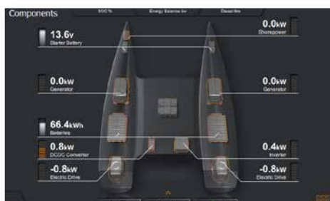
System management: Provides status data on all system components. Select individual components for more detail.
